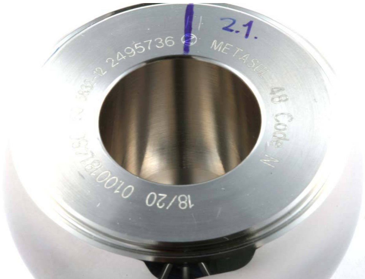
Fig. 26: Femoral head 2.1 after 2.5 million cycles. The anterior position is orientated to the left side of the picture.
