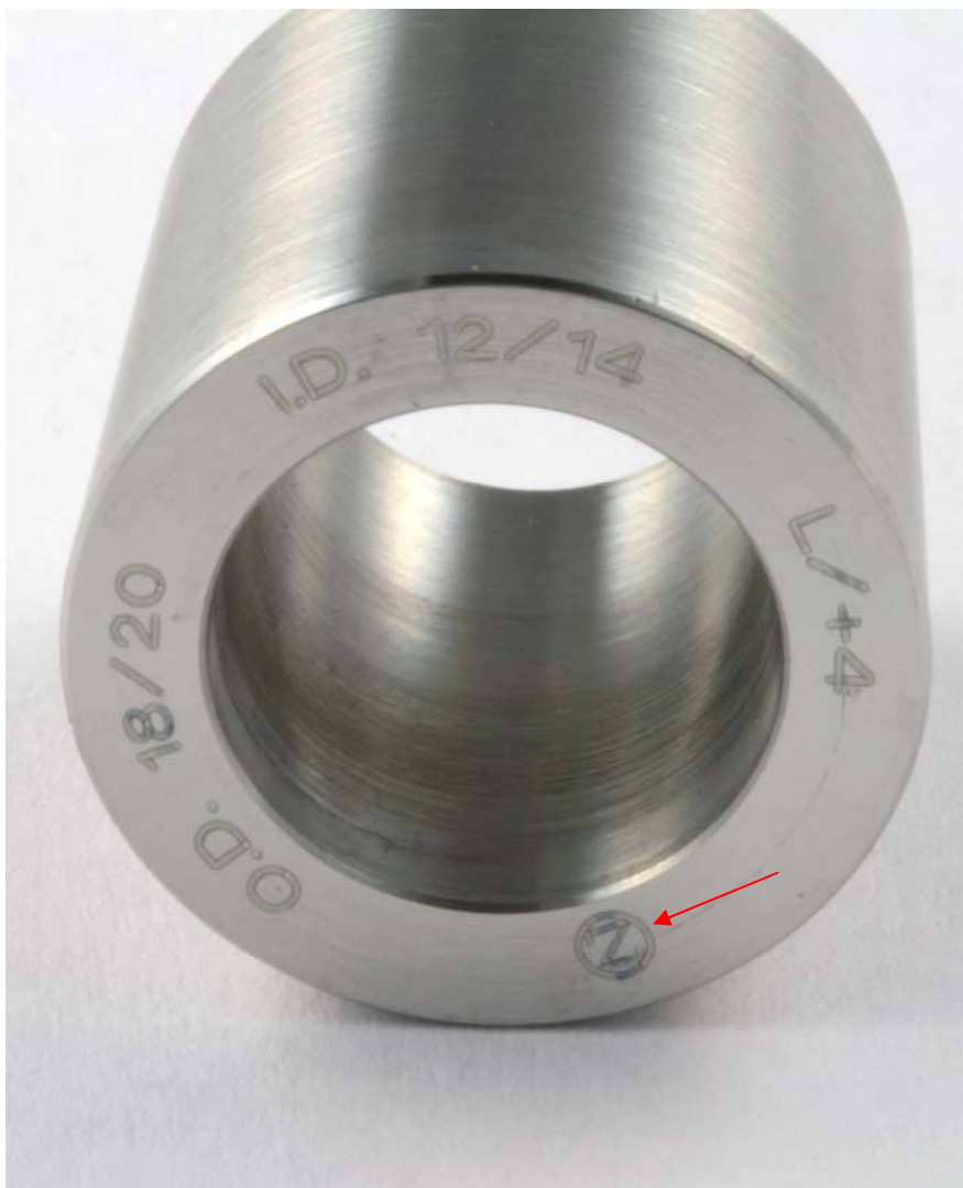
Fig. 17: Head adapter 1.1. Contact surface femoral stem side. (The red arrow marks location A, see Fig. 15)
