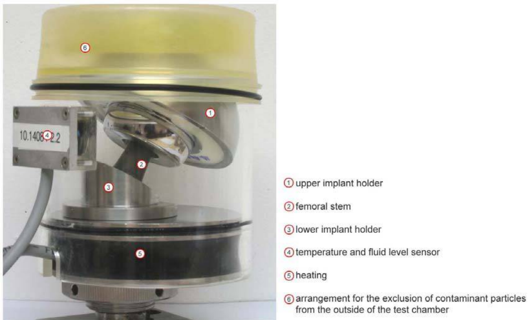
Fig. 6: Single test chamber.
