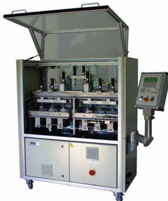
Fig. 4: EndoLab® six station hip simulator according to ISO 14242-1.
