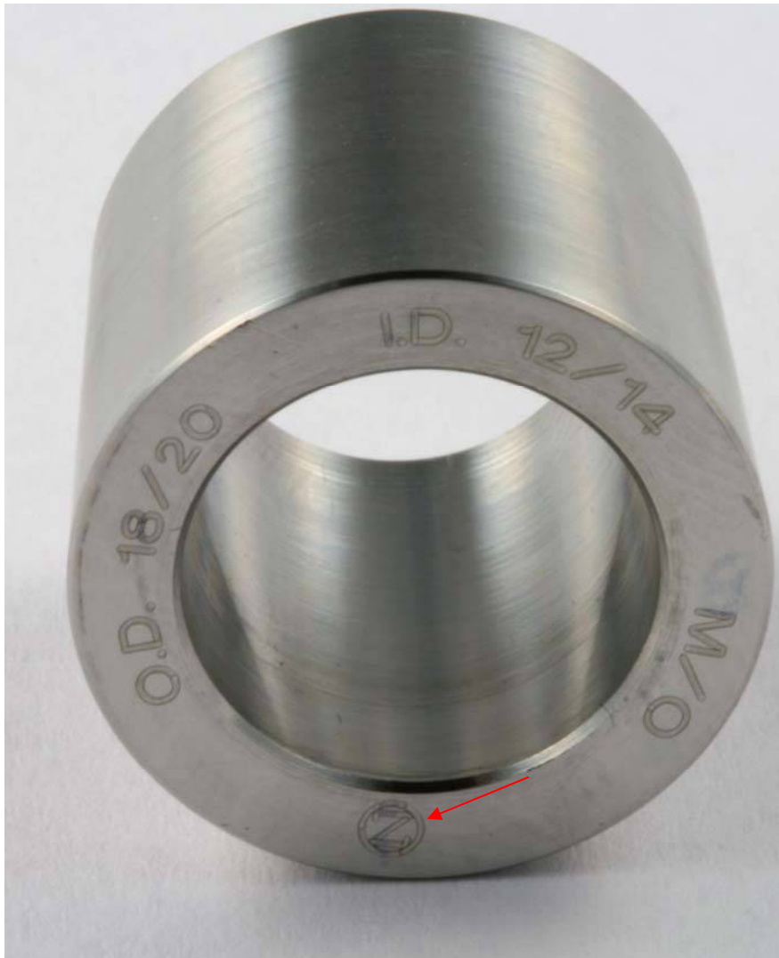
Fig. 19: Head adapter 2.1. Contact surface femoral stem side. (The red arrow marks location A, see Fig. 15)
